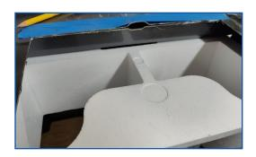
8. From inside the vehicle, lay the Styrofoam on the surface and mark the cutouts in the Styrofoam duct to fit the smaller area you are trying to fit. (You may encounter some obstructions, such as roof rails.) Keep in mind that you are adding extra inches between the unit and the internal face of the unit, so the Styrofoam needs to be adjusted on its depth measures as well.
