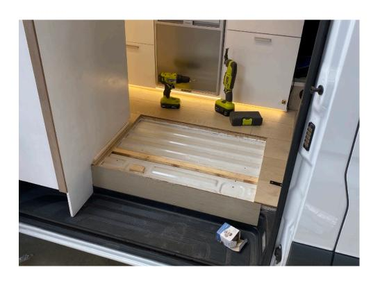
**Step 3:** Remove the drain from the shower pan and place the pan into your new cut hole.
