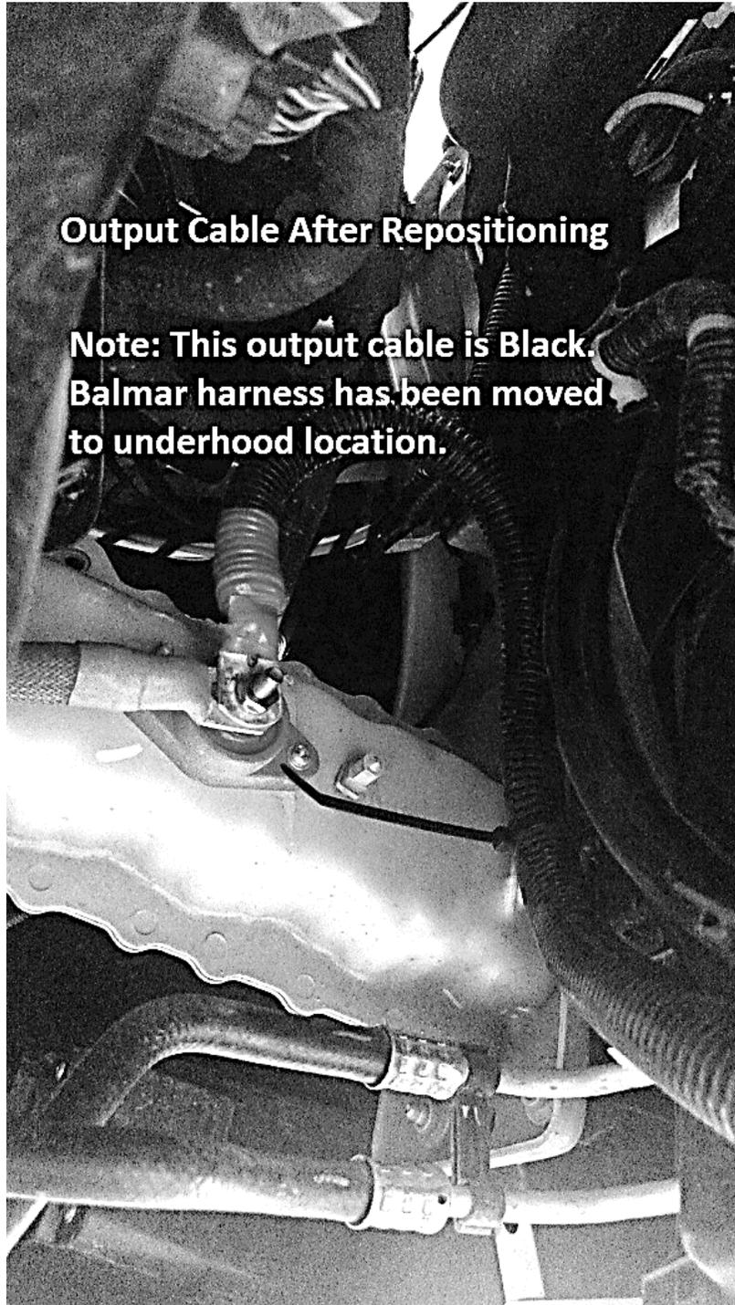
Lastly, in the factory position, the Balmar harness may or may not interfere with the E-Guard side plate. Reposition the harness as necessary to avoid interference with the E-Guard or transmission cooler lines.
