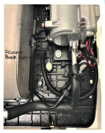
NOTE EXACT POSITION FOR THE HOLE TO MOVE POWER CORD INSIDE A VAN ETC.
