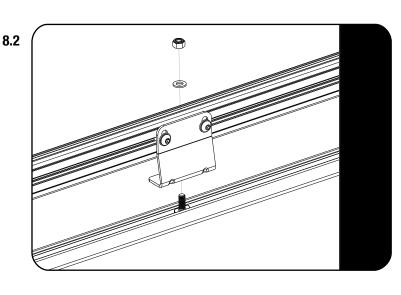
Place pre-assembled Side Profiles over the vehicles OEM tracks. Align feet with M8 x 20 T-Bolts (RRAC907) and secure the feet to the roof using M8 x 20 T-Bolts, M8 x 16 Flat Washers and M8 Nyloc Nuts. You will need a friend to help. Fully tighten.
