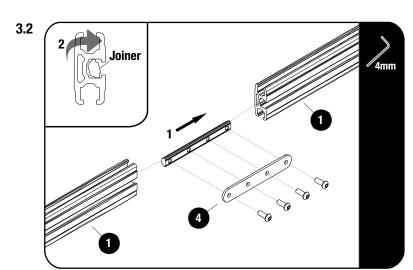
Place Joiner into the Side Profile and twist into position as shown.
