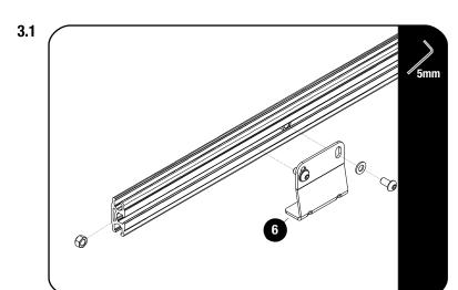
Loosely assemble the Mercedes Sprinter Feet (Item 6) using M8 x 16 Button Head Bolts, M8 Flat Washers and M8 Nyloc Nuts and slide them into the Side Profiles. They must still slide freely.
