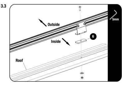
Apply Sealant around all mounting holes in the roof.
