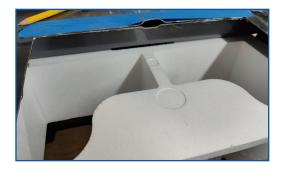
8. From inside the vehicle, lay the styrofoam against the ceiling and mark the cutouts in the styrofoam plenum needed to fit the area you are trying to fit. (You may encounter some obstructions, such as roof rails.) Bear in mind that the styrofoam plenum will be seated against the internal roof of the vehicle rather than against the external unit as it would be in a standard installation. This may require cutting down the plenum so that the vent cover reaches the mounting bolts.
