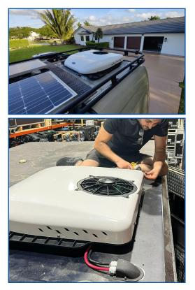
12. From inside the vehicle, you will have the unit in position and ready to install the mounting brackets provided. If necessary, adjust the brackets to distribute the load on the roof surface Don't exceed more than 15Nm torque.
