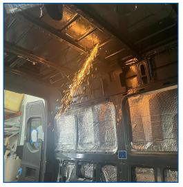
Once the opening is cut you must smooth the edges and paint it with anti-rust paint.
