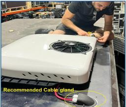
9. From inside the vehicle, you will have the unit in position and ready to install the mounting brackets provided. If necessary, adjust the brackets to distribute the load on the roof surface. Don't exceed more than 15Nm torgue.
