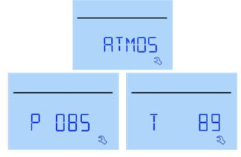
Use the rotary button to switch between atmospheric pressure and ambient temperature.
