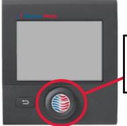
Rotary Button / Turn Knob Press and hold for 3 seconds to turn off
