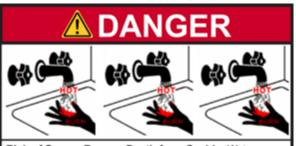
**Risk of Severe Burn or Death from Scalds.** Water temperature over 51°C (123.8°F) can cause severe burns instantly or death from scalds. See instruction manual before setting temperature at water heater. Feel water before bathing or showering. Temperature limiting valves are available, see manual.
