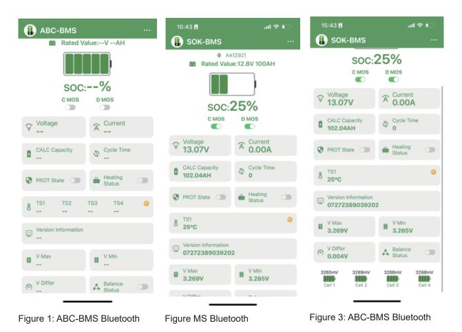
×SOC and Capacity maybe incorrect prior to cycling the battery. We suggest supplementing the app's State of Charge (SOC) with an external shunt. The app is best for checking the cell voltage and protection state information.
