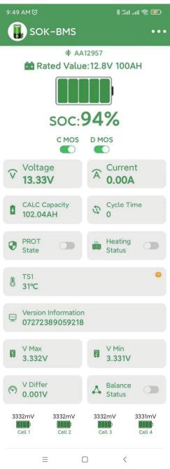
Figure 4 shows ABC-BMS home page. This page shows basic information about the connected battery, like voltage, current, individual cell voltage, software version, etc.
