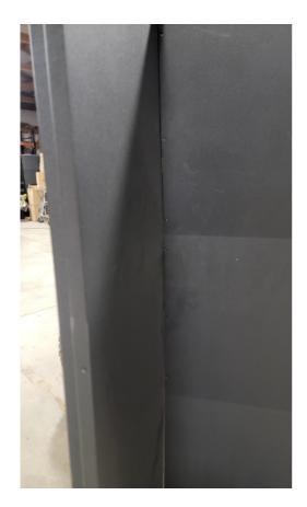
Place the 5/8" tab of the right side behind the rear panel and repeat the same process with 10 more rivets.
