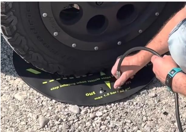
Image 11: Connecting the air pump
