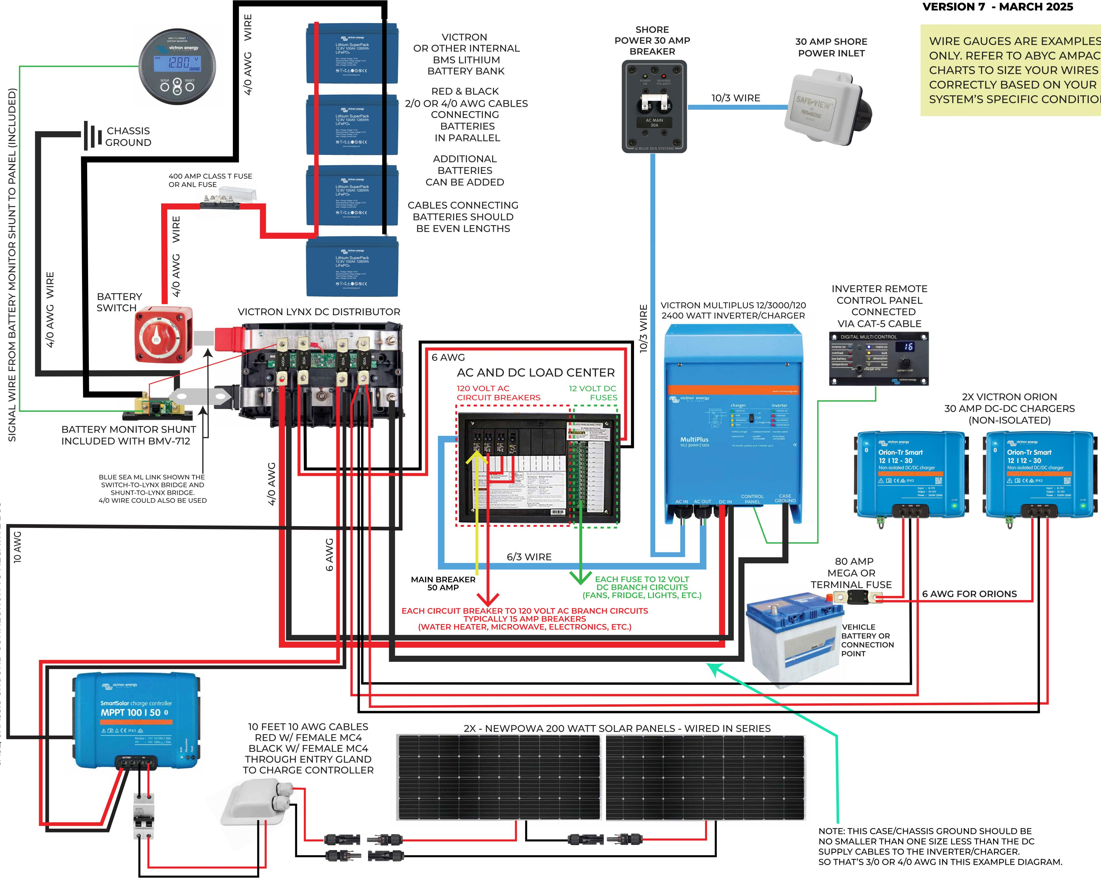
WIRE GAUGES ARE EXAMPLES ONLY. REFER TO ABYC AMPACITY SYSTEM'S SPECIFIC CONDITIONS
